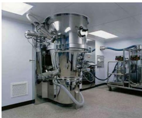
Figure 3: Fluid bed top spray granulator
