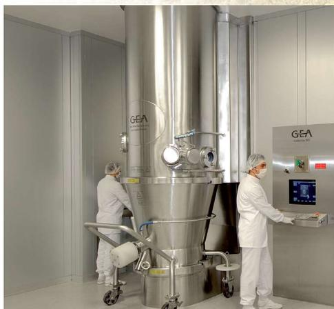
Figure 2: FlexStream™ fluid bed processor
