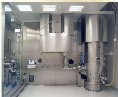
Figure 4: A typical integrated production line for pharmaceutical granules
