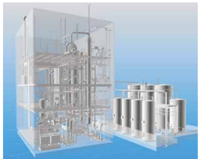
Distillation plant for the recovery of solvents from a wet spinning process in a chemical fiber production plant
