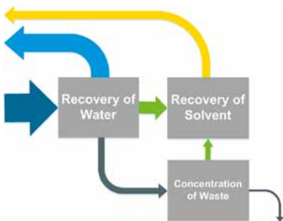
Mass flow diagram of the different process streams in a solvent recovery plant for aqueous solutions
