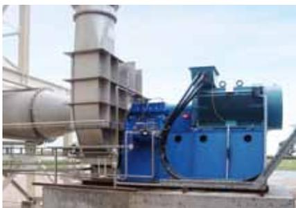
shape. After having passed the impeller, the vapour is conveyed in the spiral housing to the discharge nozzle where it is discharged from the machine at a higher pressure and temperature level.
