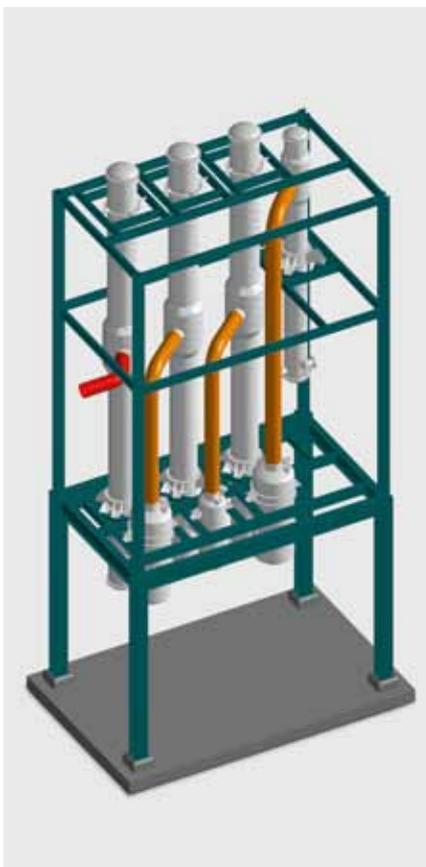
*Before: Three-effect falling film evaporation plant, directly heated*
