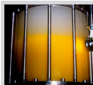
The wash column (ice separator) of a commercial Freeze Concentration plant for orange juice illustrating the sharp separation between washed ice (top) and ice with concentrate (bottom).
