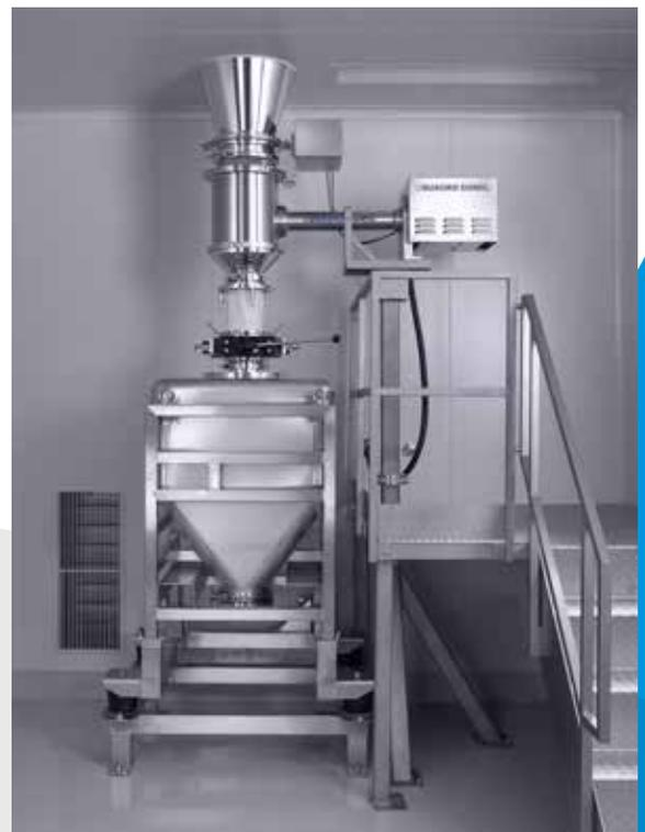
*Production scale contained discharge system including milling option*
