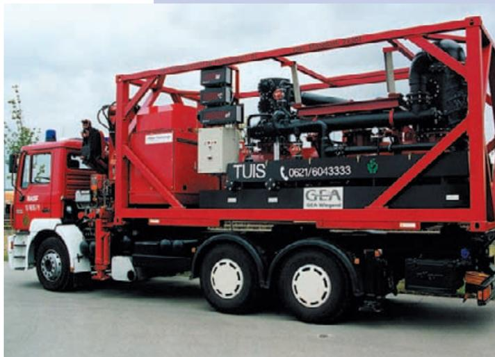
*Mobile chlorine emergency unit in operation*
