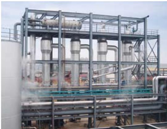
4-effect falling film evaporator with thermal vapour recompression for lysine solution with stripping column for  $\text{NH}_3$  separation and condensation
