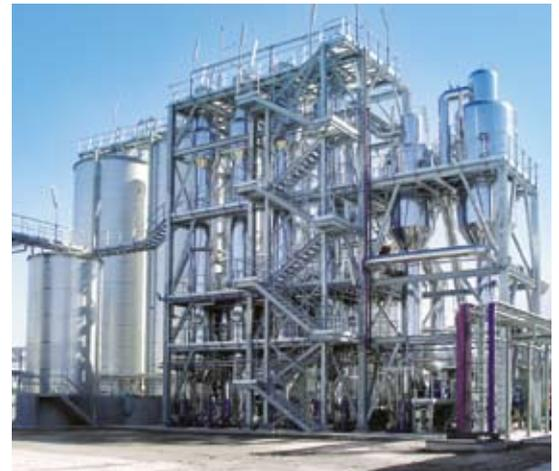
4-effect falling film/forced circulation evaporation plant with thermal vapour recompression for fermentation waste water
