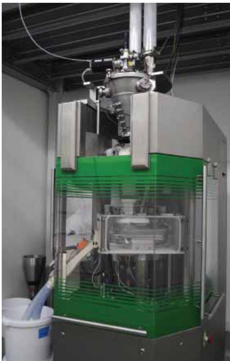
in conventional presses. By measuring and combining these two signals, tablets with a deviating pellet concentration can be detected.
