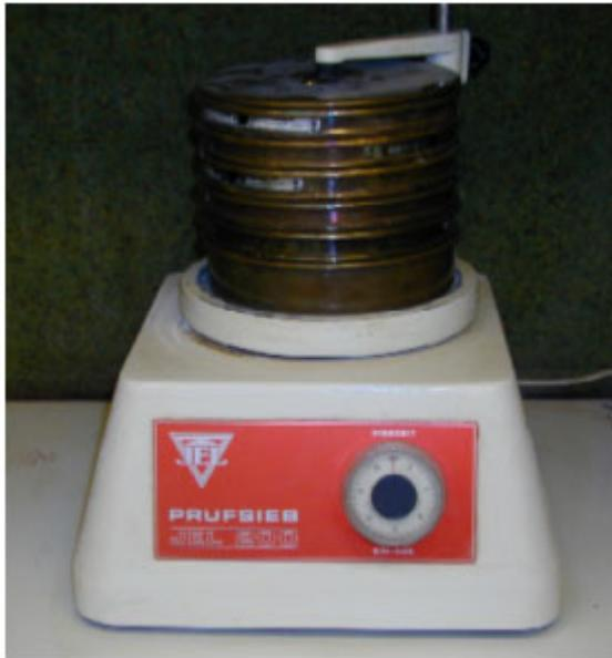
Fig. 1 Shaker for sieves.
