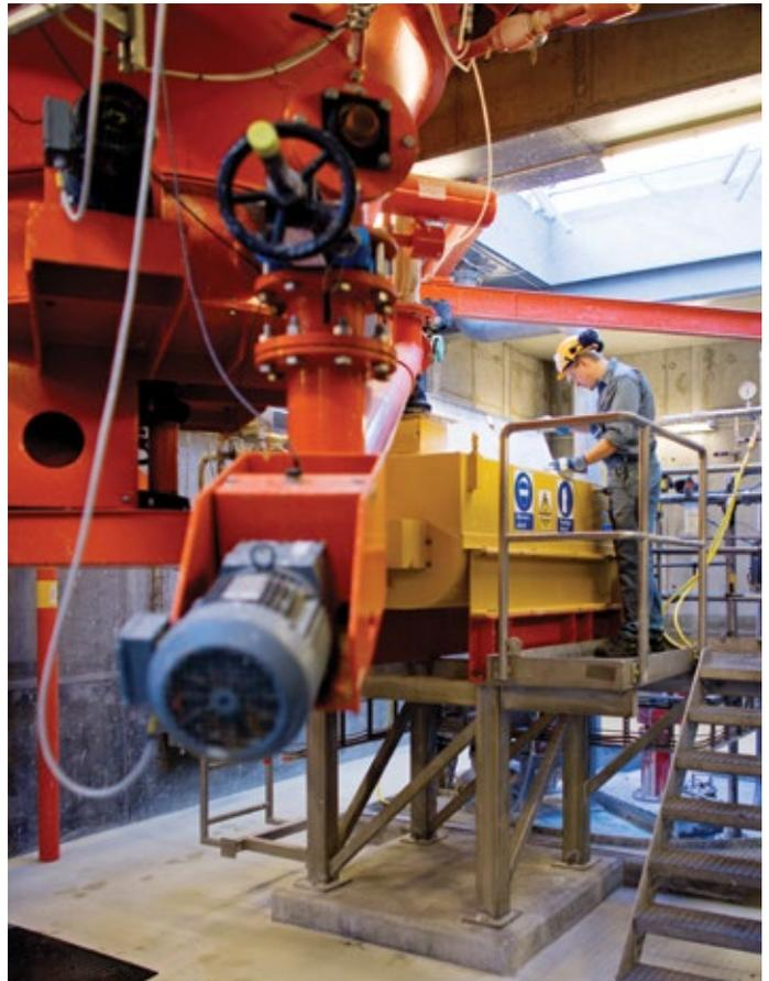
*Erection of a gas disperser at a German incineration plant.*
