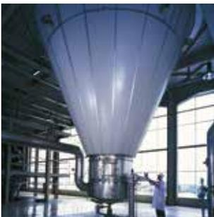
*Fluidized spray dryer - FSD™ with integrated fluid bed*
