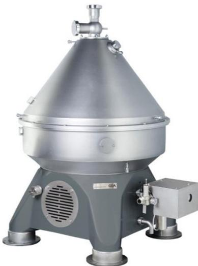
**Pic. 1:** [GEA clarifiers for miscella clarification have a gas-tight design with nitrogen blanketing for reliable explosion-protection. \(Pic. GEA\)](#)
