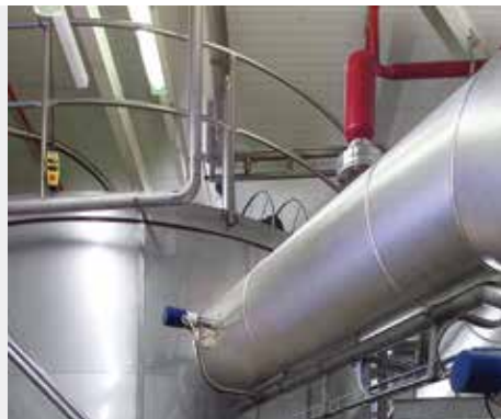
GEA Niro Spray dryer - side view
