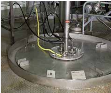
GEA Niro Spray dryer - top view
