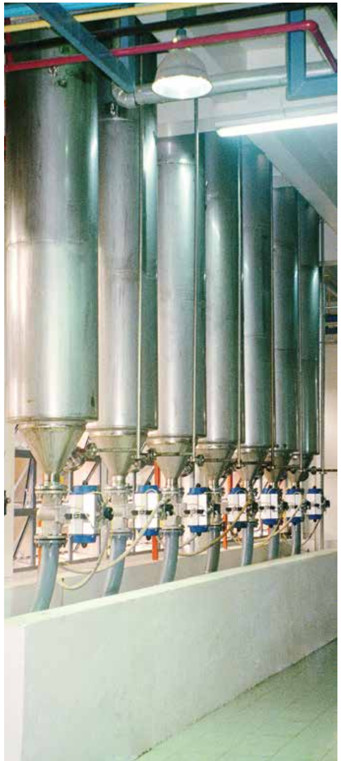
Conventional batch percolator - bottom view
