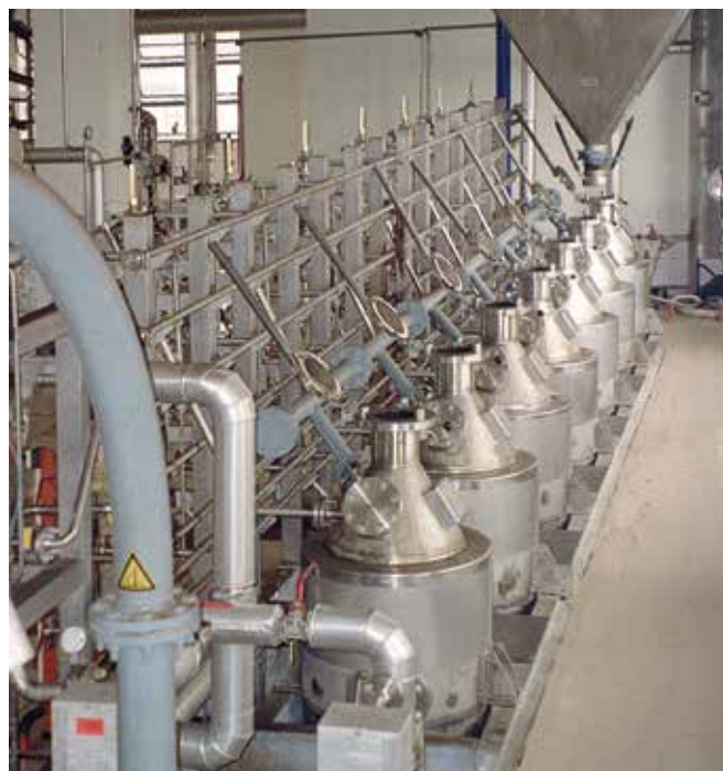
Conventional batch percolator – top view
