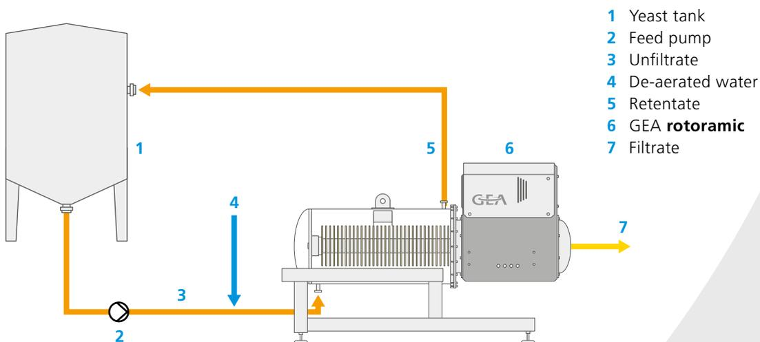
Figure 4 – Flow chart of the GEA rotoramic beer recovery
