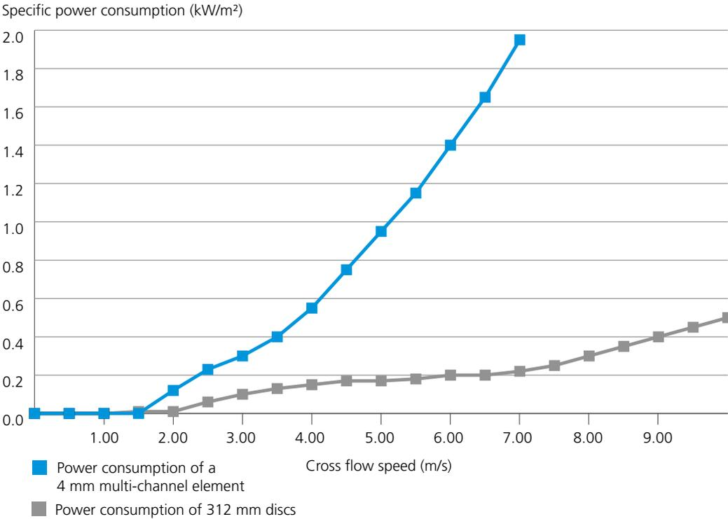
Figure 7 – Comparison of energy consumption
