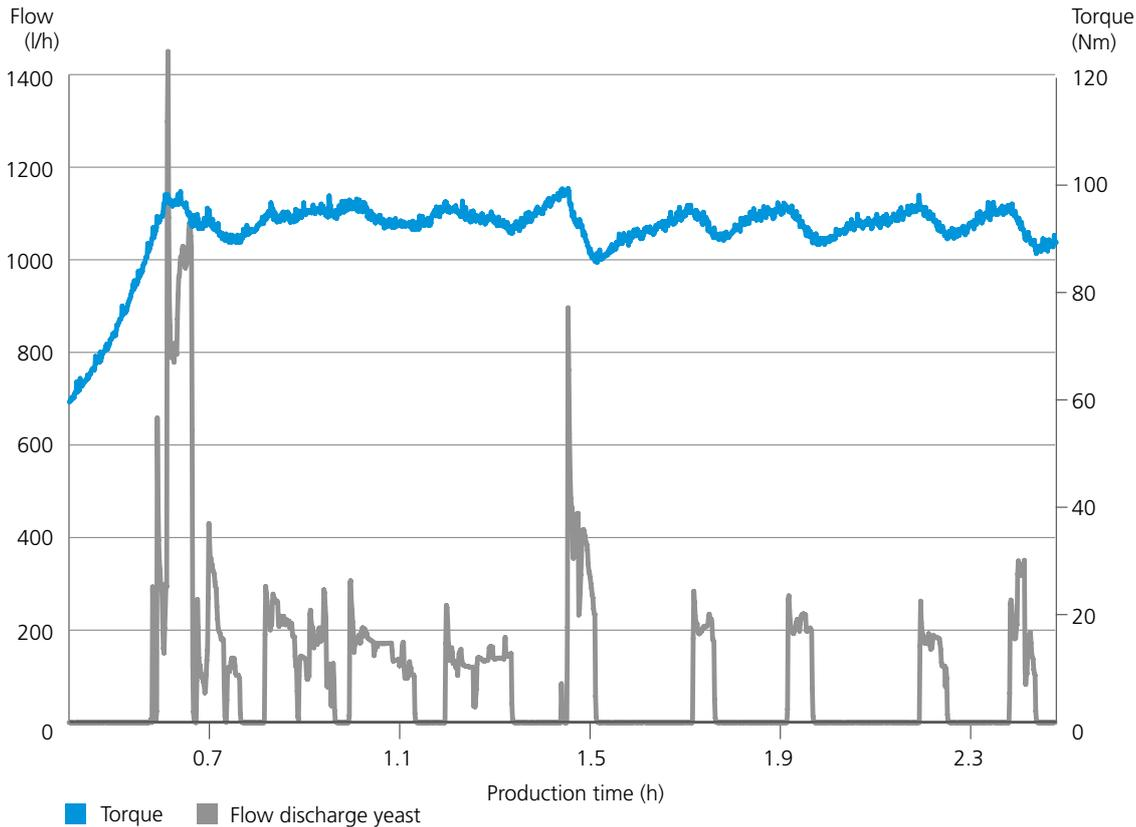
Figure 6 – The effect of torque on the discharge flow of yeast
