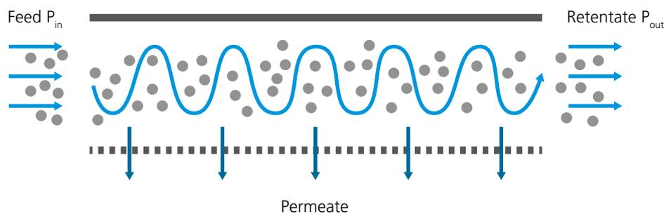
Figure 1 – Principle of cross-flow filtration
