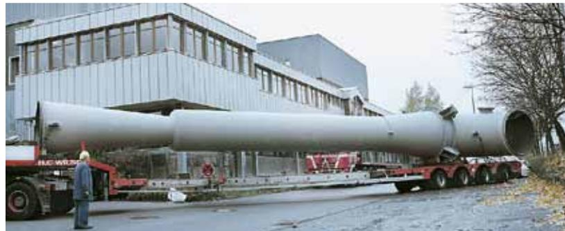
*Jet pump for a 4-stage jet vacuum pump for steel degassing
