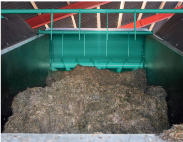
Beater rollers: ensure an even and precise dosage
