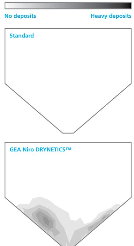
*The superiority of GEA Niro DRYNETICS™ as a predictive tool is clearly shown in this comparison. Standard software fails to detect the accumulation of sticky deposits on the dryer's walls, whereas GEA Niro DRYNETICS™ pinpoints the problem, suggesting the need for a redesign or operational improvement.*
