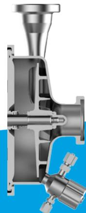
Figure 1: Drain valve
