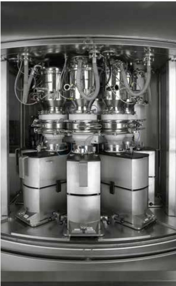
*GEA Compact Feeder arrangement in the CDC 50 for direct compression*
