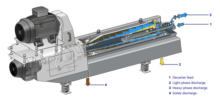
When the solids content in the suspension to be processed is higher than 2% it is time to call in the decanters. They are often placed upstream of a disk stack centrifuge and achieve high clarification efficiencies and maximum dewatering.
