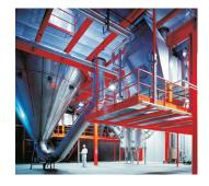
Spray Drying Evaporation (SDE), for achieving zero liquid discharge (ZLD). The heat source for effluent evaporation can be hot flue gas or pre-heated combustion air.
