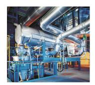
Small-scale spray dryers for product testing and production, available in different configurations and sizes, also in closed-cycle design which enables solvent recovery.
