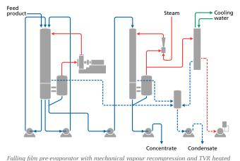
Falling film pre-evaporator with mechanical vapour recompression and IVK heated finisher in special design for coffee extract.
