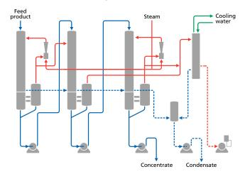
Falling film pre-evaporator with thermal vapour recompression and TVR heated finisher in special design for coffee extract.
