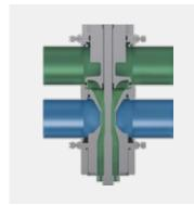
If there is cleaning media in the upper pipeline, the upper valve disc can be lifted up to allow the surface of the seal and the leakage chamber to be cleaned.
