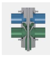
If there is cleaning media in the lower pipeline, the lower valve disc can be lowered downward to allow the surface of the seal and the leakage chamber to be cleaned.
