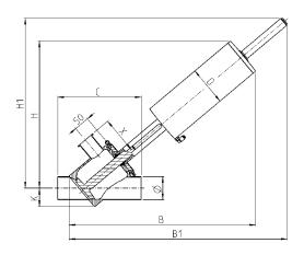
Angle Valve with CIP Connection
