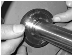
MF-587 Fig. 42: V-ring on pump side
