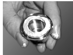
Fig. 75: Nord-Lock washer in impeller nut
