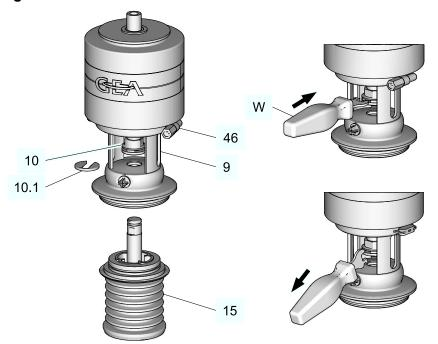
Fig.14: Removing the bellows
