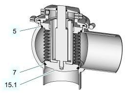
Fig.6: Design of metal bellows
