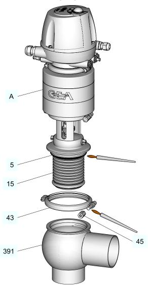
Fig.29: Installing the valve
