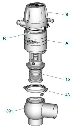
Fig.13: Valve insert
