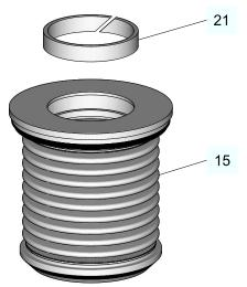
Fig.24: Changing the guide ring of the metal bellows
