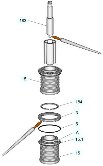
Fig.26: Mounting the PTFE bellows
