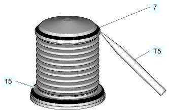
Fig.21: Removing the V-ring
