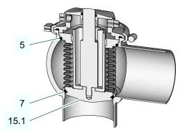
Fig.19: Replacing wearing parts of valve with metal
