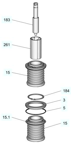
Fig.15: Dismantling the PTFE bellows
