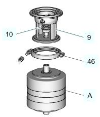
Fig.16: Dismantling the lantern
