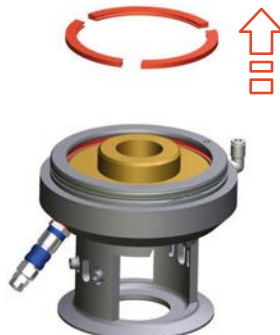
Fig.100: Removing securing elements
