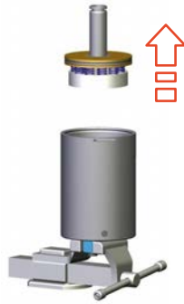
Fig.97: Lifting out top spring assembly
