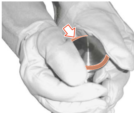
Fig.84: Mounting the valve seat seal
