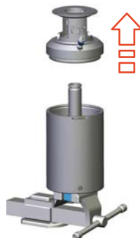
Fig.96: Removing actuator base
