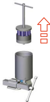
Fig.98: Lifting out bottom spring assembly
