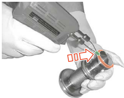
Fig.81: Cut through valve seat seal
