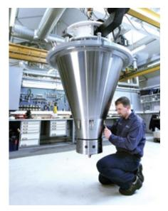
In particular, stripping of VOCs from dry polymers is a growing requirement. It could well become a general processing standard, due to concern about the release of VOCs during handling, storage and fabrication. The GEA Niro dryers can include both integrated and separate stripping stages. Stripping of VOCs is a special form of heat treatment/drying often performed in specially designed Stripper Fluid Beds.
