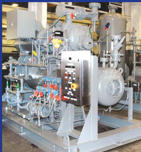
Ammonia compressor package Model 235S; 450 HP
