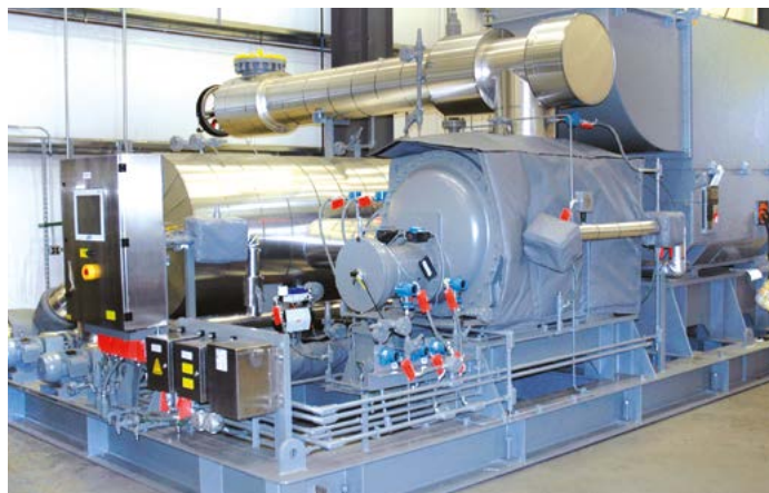
Mixed-gas compressor package Model 1640S; 2,670 HP
