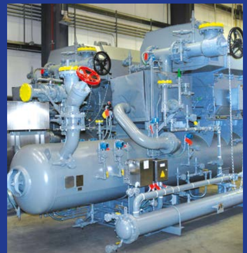
Ammonia BOG compressor package Model 565GL; 872 HP
