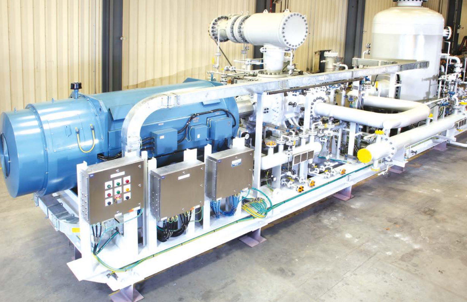
Propane refrigeration compressor package Model 1920S; 2,700 HP
