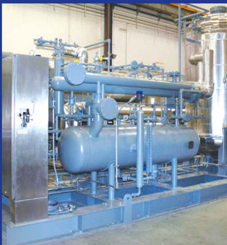
Ammonia condensing unit Model 1435GL; 1,750 HP
