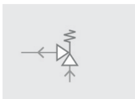
Fig.63: Oil pressure regulating valve
