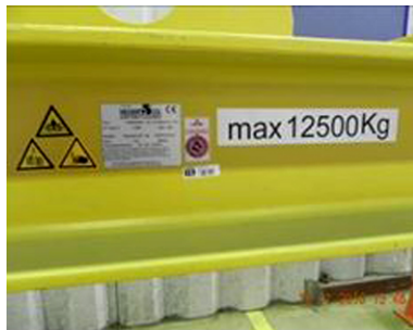
Fig.38: Example - load handling equipment weight marking
