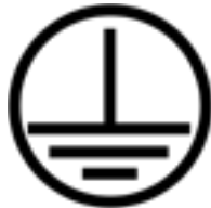
Fig.25: Designation of the earthing connection
