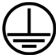
Fig.25: Designation of the earthing connection
