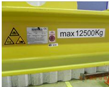
Fig.39: Example - load handling equipment weight marking
