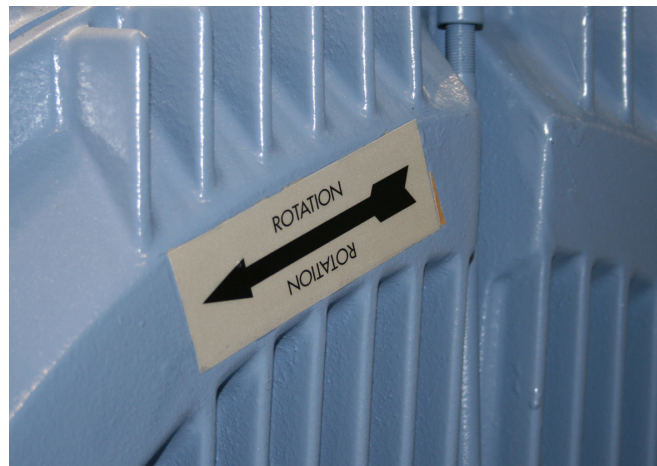
Fig.20: Marking of direction of rotation of the compressor drive motor
