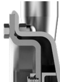
O-ring sealing between pump housing and cover
