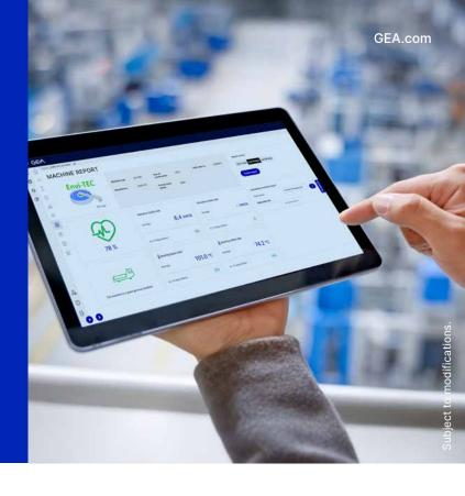
**GEA InsightPartner® Separation Monitoring**, the online condition monitoring for GEA centrifuges, includes continuous tracking of machine asset parameters such as vibrations and bearing conditions using data analytics and additional sensors\*. The system visualizes real-time and historical data, enabling early detection of potential issues, timely maintenance and reduced downtime.
