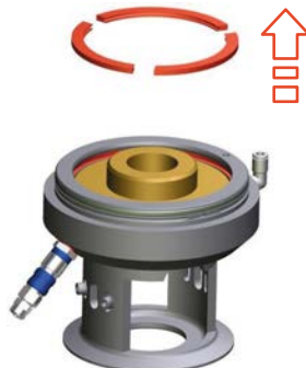
Fig.115: Removing fuse elements
