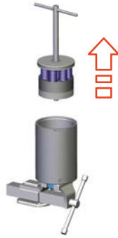
Fig.113: Lifting out bottom spring assembly
