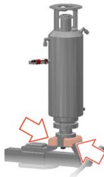
Fig.108: Clamping the actuator
