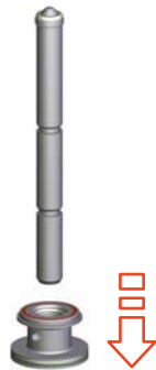
Fig.85: Pull off the bottom part of the actuator
