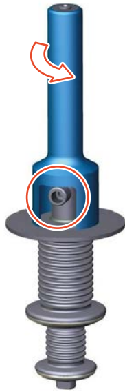
Fig.104: Align opening with the leakage socket
