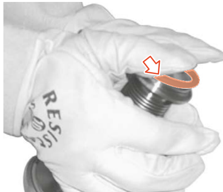
Fig.98: Place the valve seat seal into the groove
