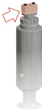
Fig.107: Attaching clamping piece
