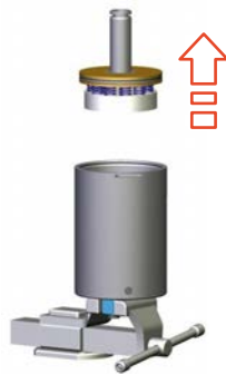
Fig.112: Lifting out top spring assembly
