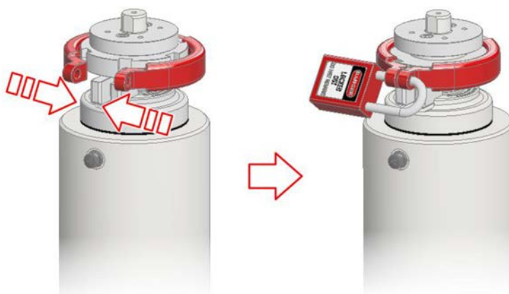
Fig.20: Lock the locking mechanism
