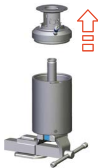
Fig.111: Removing actuator base
