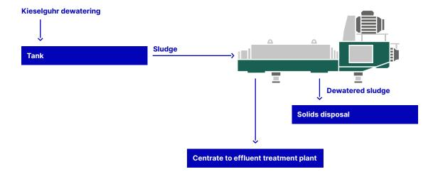
The spent Kieselguhr slurry is collected and conveyed to the decanter centrifuge by a screw pump. The decanter separates the Kieselguhr from the liquid. The dewatered Kieselguhr is then collected in a container for disposal. The reduced amount of waste saves disposal and transportation costs. In addition, the Kieselguhr-free fluid is now easier to process in a wastewater treatment plant.
