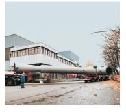
Three-stage steam jet cooling plant in bridge design. Cooling of 194 m3/h of water from 28 °C to 1 °C. Refrigeration capacity: 2,900 kW
