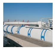
Ejector for a four-stage steam jet vacuum system for steel degassing. Suction flow rate: 1,100 kg/h (1,387,000 m<sup>3</sup>/h) from 0.6 mbar.
