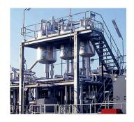
Draft Tube Baffle Crystallizer (DTB):
