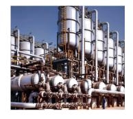
Forced circulation evaporator: Ideal for highly viscous liquids or with a tendency to form incrustations. Optimal for inorganic solutions among other applications.
