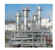
CompaCon® Evaporator: Skid-mounted falling film and forced circulation evaporators for small-scale production. Energy efficient, easy to transport and assemble.
