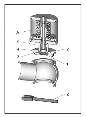
⇒ Valve insert has been dismantled into its individual parts.
