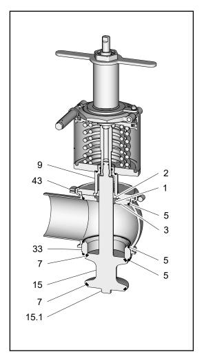
⇒ The valve insert is assembled from individual parts.
