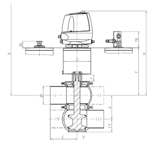
Fig.1: valve W\_/ECO with control top T.VIS
