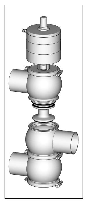
⇒ The valve insert has been installed.
