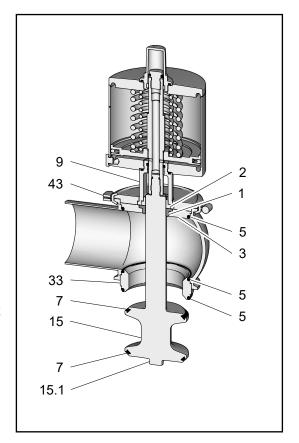
⇒ The valve insert is assembled from individual parts.
