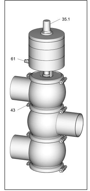
⇒ The clamp connection between the upper and middle housing has been dismantled.
