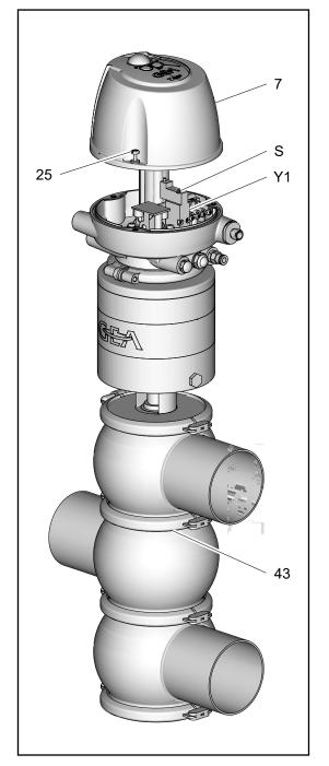
3. Remove hinged clamps (43) between the upper and middle housing.
