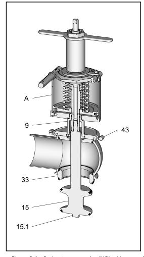
Figure 9-1 - Spring-to-open valve (NO) with manual emergency actuator
