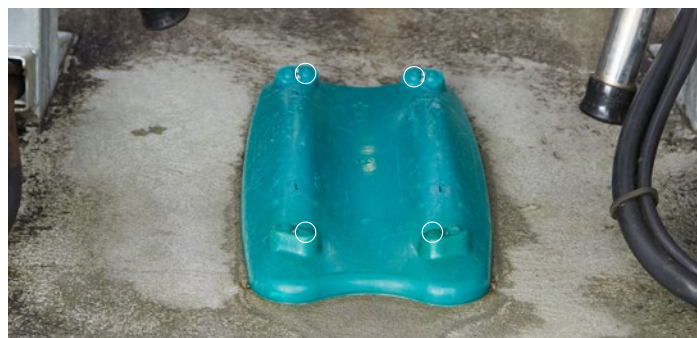
Post-spray nozzles set closer together for milked-out udders, where teats are positioned closer together.
