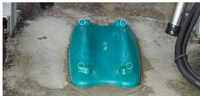
Pre-spray nozzles set wider apart for milk-filled udders, where teats are set further apart.
