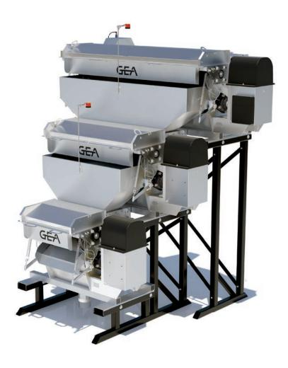
XPress<sup>™</sup> 6FT - 4FT - 2FT with integrated regulator tank Shown with high stand for XPress<sup>™</sup> 6FT and two-level stand for XPress<sup>™</sup> 4FT and 2FT
