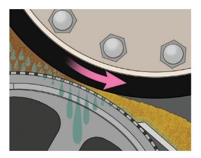
The XPress<sup>™</sup> rotation pulls in a steady stream of material from the integrated regulator tank or dewatered material from a sloped screen or vertical dewaterer. The fiber material is squeezed between an upper rubber roller and a lower stainless steel screen to remove moisture. The extracted liquid is diverted from the fiber material via openings in the screen roller. The process is repeated two or three times depending on the capacity or dry matter rate targeted.
