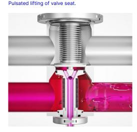
**4. SIP steam flush both valve seats** Rinse of steam via leakage chamber. Pulsated lifting of valve seat.
