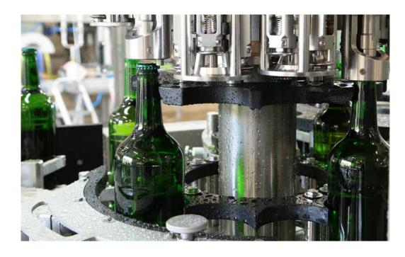
Different bottle types use different closures, so we've made sure that the Visitron Filler G can handle a diverse range of caps, including alu-screw caps, crown corks and PCO caps. The open design of the cappers means that the equipment can be easily and thoroughly washed.
