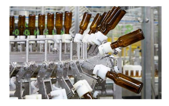
All containers need to undergo rinsing before filling to remove dust, dirt, and other potential contaminants. The Visitron Filler G machines are compatible with a wide range of rinsing media, including ionized air, sterile water, disinfectant, or alcohol. We can also configure an optional water or disinfectant recirculation system that saves on water or disinfectant usage, and so reduces costs and waste.
