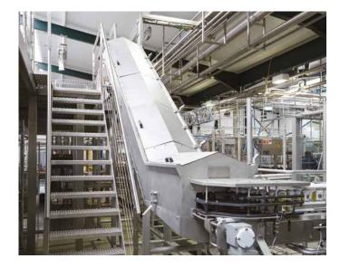
Before filling, each container must be rinsed to remove dust, dirt and other potential contaminants. The Visitron Filler C filler/seamer units can be equipped with either a classic gravity rinser, or a rotary version. The rotary rinser is compatible with a wide range of rinsing media, and feature nozzles that are designed to ensure that the entire internal surface of every container is reached. This increases efficiency and saves resources, without wasting media.
