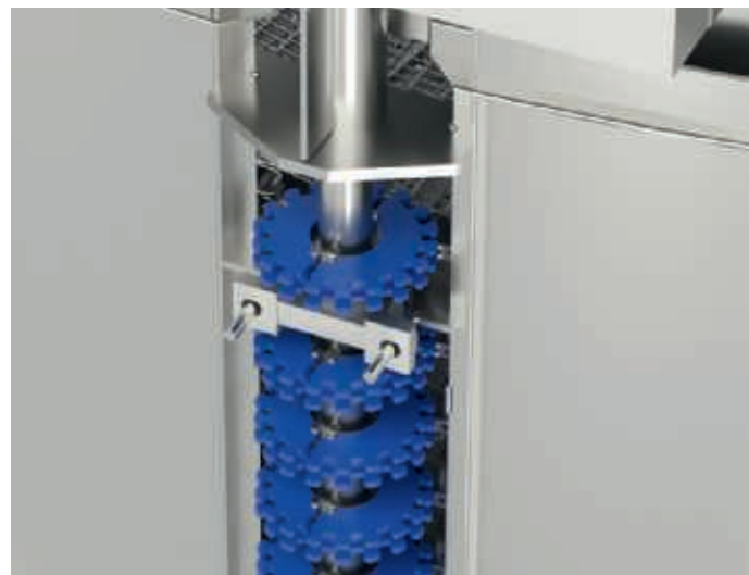
The GEA ProEdge system drives the spiral conveyor belt from its outside edge. Sprockets at each spiral tier level engage into belt links, and the two sprocket shafts are driven by synchronized motors.
