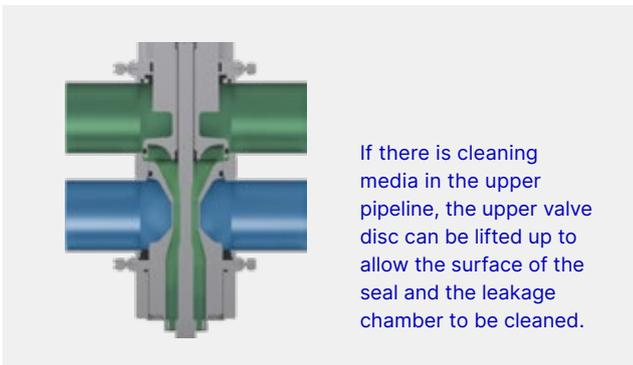
In this case, the cleaning media passes the seal of the lifted valve disc, cleans the leakage chamber and then flows out through the leakage outlet into the periphery. Therefore, it is possible to clean all surfaces that come into contact with the product, including the seal surfaces of the valve disc seals.
