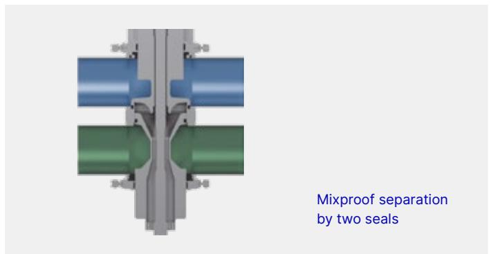
When the valve is closed (non-actuated position), there are always two seals between the separated pipelines. If one seal is defective, the resulting leakage will be directed through the leakage outlet into the periphery, without mixing with the product in the second pipeline.
