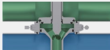
If there is cleaning media in the upper pipeline, the upper valve disc can be lifted to allow the surface of the seal and the leakage chamber to be cleaned.
