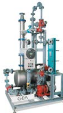
Compact gas scrubber KGW DN80 W for 50 m 3 /h exhaust gas containing 1 kg/h Cl 2 . Materials: steel/PTFE and stainless steel/ECTFE
