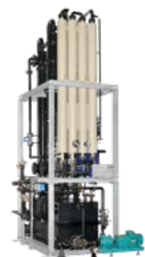
Compact gas scrubber KGW for exhaust gas containing EO/PO (ethylene oxide and propylene oxide) during tank and pipeline work Separation efficiency 99.999 %, clean gas value 0.5 mg/Nm 3 EO/PO
