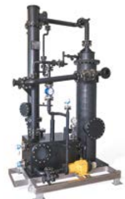
Compact gas scrubber KGW DN80 with aerosol separator for 7 m 3 /h exhaust air containing chlorine compounds. Materials: PP EL, frame of stainless steel
