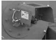
Safety guard for power take off driveline (American model) (Part No. 2018-7603-040)
