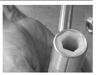
Fig.54: Socket wrench with insert
