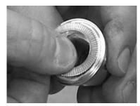
Fig.51: Lock washers in impeller
