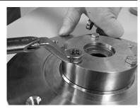
Fig.25: Seal cartridge
