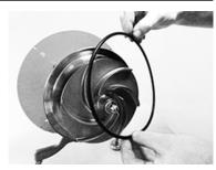
Fig.57: Back plate, O-ring
