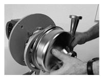
Fig.58: Annular casing
