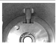
Fig.29: Seal cartridge
