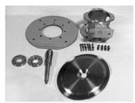
Fig.19: Pump shaft and motor stool
