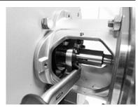
Fig.33: Clamp connection
