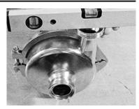
Fig.60: Annular casing
