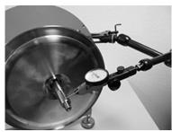
Fig.34: Measuring the pump shaft
