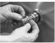
Fig.40: Seal spacer
