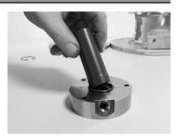
Fig.21: Radial packing ring
