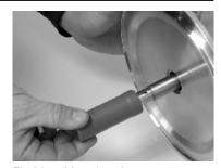
Fig.31: Mounting sleeve
