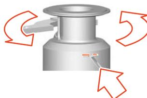
Fig.89: Fixer le ressort de montage
